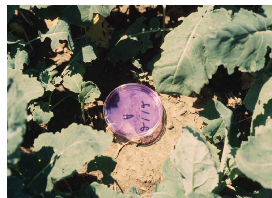
Figure 2. Steadman test used to estimate SSR risk.
